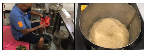
Figure 8: Mixing process by hand held motor driven by agarwood-inducing mixing machine Figure 9: Mixing process by agarwood-inducing inoculum mixing machine
